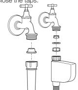
Remove the nuts of the water intake hoses to clean the surfaces of the filters on the water intake valves with an appropriate brush.
